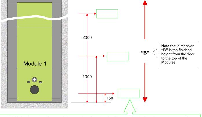
To ensure that the supplied Module fits neatly and accurately between the walls and to allow for any vertical deviation between the wall surfaces, please provide the horizontal distance between the walls at the three heights indicated, i.e. 150mm, 1000mm and 2000mm from the floor level.
