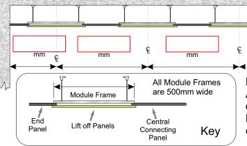
Note that dimension **A** is the depth of the duct enclosed by the Modules and cannot exceed 250mm.
