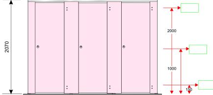
To ensure that the supplied kits fit neatly and accurately between the walls and to allow for any vertical deviation between the wall surfaces, please provide the horizontal distance between the walls at the three heights indicated, i.e. 150mm, 1000mm and 2000mm from the floor level.
