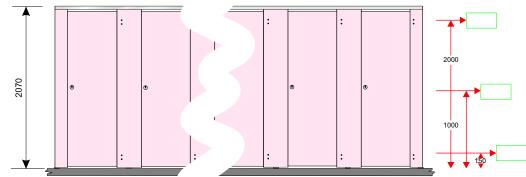
To ensure that the supplied kits fit neatly and accurately between the walls and to allow for any vertical deviation between the wall surfaces, please provide the horizontal distance between the walls at the three heights indicated, i.e. 150mm, 1000mm and 2000mm from the floor level.
