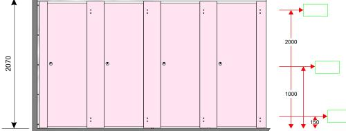
To ensure that the supplied kits fit neatly and accurately between the walls and to allow for any vertical deviation between the wall surfaces, please provide the horizontal distance between the walls at the three heights indicated, i.e. 150mm, 1000mm and 2000mm from the floor level.
