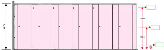
To ensure that the supplied kits fit neatly and accurately between the walls and to allow for any vertical deviation between the wall surfaces, please provide the horizontal distance between the walls at the three heights indicated, i.e. 150mm, 1000mm and 2000mm from the floor level.
