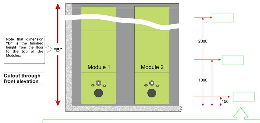
To ensure that the supplied Modules fit neatly and accurately between the walls and to allow for any vertical deviation between the wall surfaces, please provide the horizontal distance between the walls at the three heights indicated, i.e. 150mm, 1000mm and 2000mm from the floor level.
