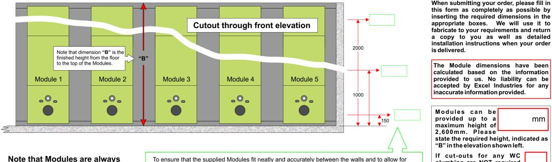
To ensure that the supplied Modules fit neatly and accurately between the walls and to allow for any vertical deviation between the wall surfaces, please provide the horizontal distance between the walls at the three heights indicated, i.e. 150mm, 1000mm and 2000mm from the floor level.
