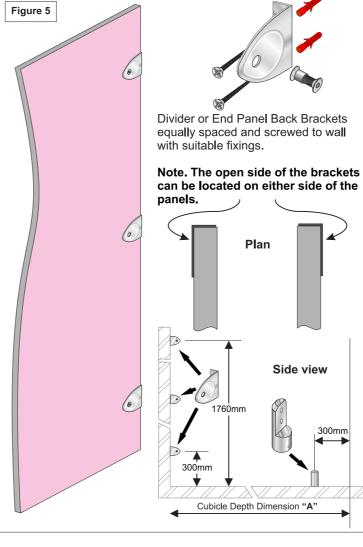
2c Whilst supporting the Panel on the timber batten at the back and on the Panel Base Support close to the front edge of the Panel, locate the panel against the Divider Panel Brackets and drill 8mm holes through the fixing holes in the Brackets and secure with the provided Tee Nuts. Then align the pre-drilled holes in the Panel with those in the Base Supports and secure with the provided Single Tee Nuts. Remove the temporary battens.
