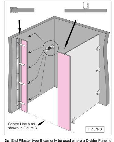
used to close off the side of any cubicle not located against a wall. It features the section of aluminium channel pre-fixed at right angles. It can be used on the left or right side of the cubicle. They are also identified with labels to ensure that they are not installed upside down where being used on the door hinge side as they are NOT handed. See Figure 9.
